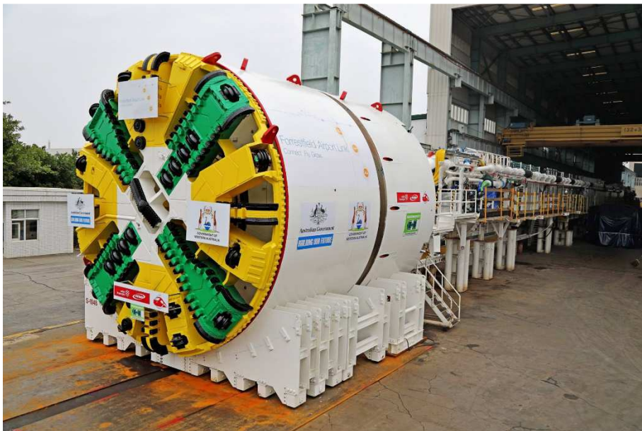
Variable Density TBM used in FAL project © www.forrestfieldairportlink.wa.gov.au
