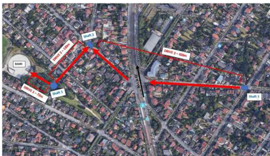
Layout of the new storm water tunnel
